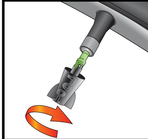
**6** Reinstall valve core.
