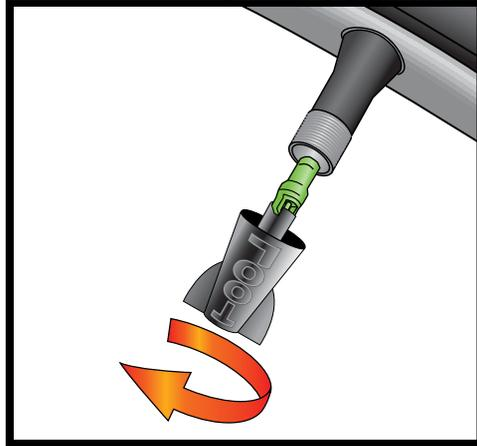
**2** Remove valve core with included tool.
