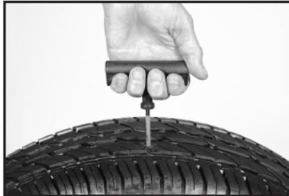
(EN) Slide the reamer tool in and out of your tyre puncture multiple times to roughen and clean the inside of the hole.
