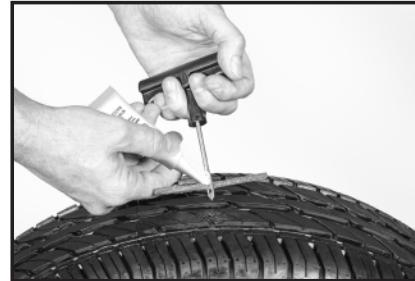
(EN) Remove a plug from its clear backing, then thread it halfway through the eye of the plugger needle. Coat the middle section of the tyre plug with Plug Bond.
