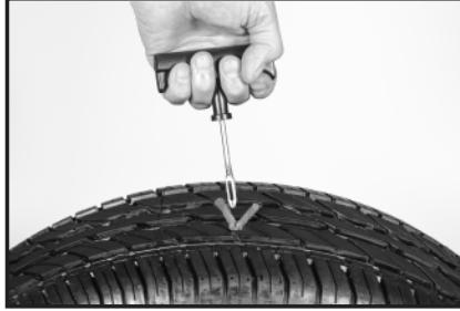
(EN) Pull the plugger tool straight out of your tyre with a rapid motion, leaving the tyre plug behind. Do not twist the needle.
