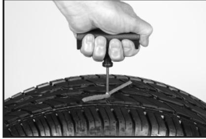
(EN) With the plug centered in the eye of the needle, start pushing the plugger tool and plug into your puncture. Stop pushing when the plug is 2/3 of the way into the hole.
