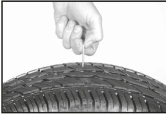
EN Inspect and remove the source of the puncture. NOTE: Some items may require the use of pliers or similar tool to remove.
