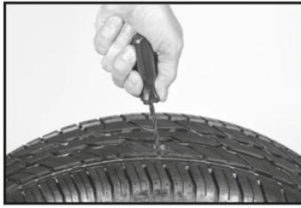
EN Insert reaming tool into hole in tyre. Using in/out motion clean out puncture to prepare for repair. Make sure to remove all debris.
