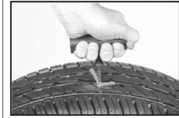
EN Using the plunger, insert the plug into the puncture making sure to leave at least 1/2" remaining above the tyre.
