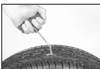
EN Remove the plunger while carefully making sure that the plug stays completely inside the puncture.
