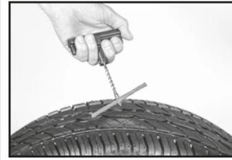
EN Remove one of the repair plugs from the package and install it onto the plunger.
