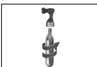
EN PREPARING THE MICROFLATE FOR USE: Lightly screw the CO2 cartridge into the threaded base of the Microflate until resistance is felt. Next, twist cartridge QUICKLY and FIRMLY, but not too tight, to puncture and seal the cartridge. The microflate is now ready to use.
