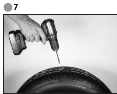
(EN) Pull the drill straight out of our tire with a rapid motion, leaving the tire plug behind. Do not twist the needle.
