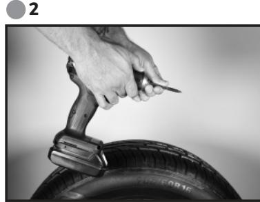
(EN) Secure the reamer bit into your drill.
