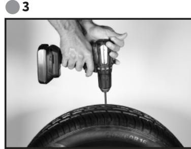
(EN) Slide the reamer tool in and out of your tyre puncture multiple times to roughen and clean the inside of the hole.
