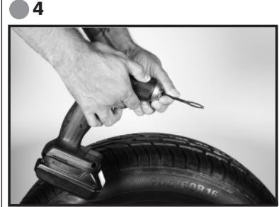
(EN) Secure the plug bit into your drill.
